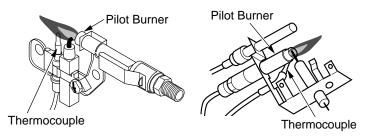
Figure 34 - Correct Pilot Flame Pattern (Your pilot may vary from pilots shown)
